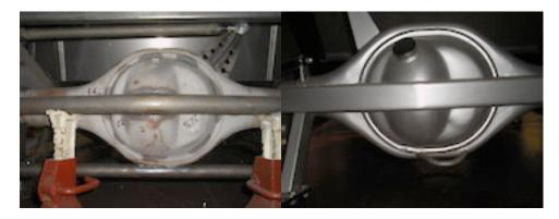
Not Accepted Housings (Rear end must NOT be fabricated or appear fabricated.)
